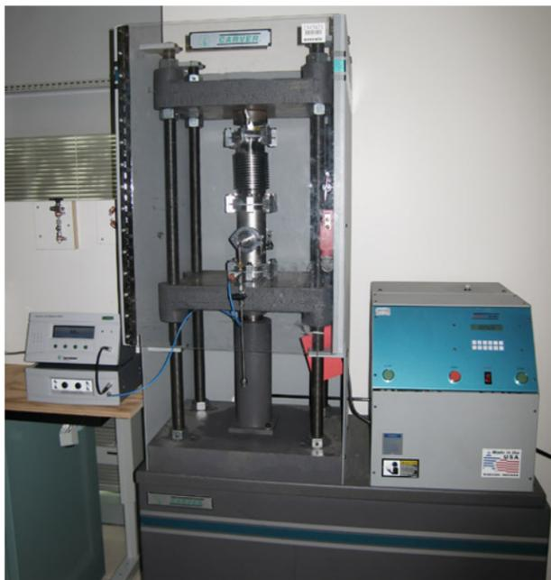
Crushing rock samples in a stainless steel chamber (center) releases the stored hydrogen molecules measured by the hydrogen detector (left).
